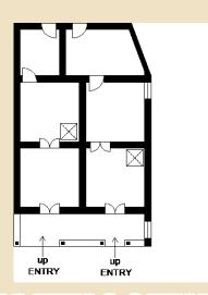
The structure is load-bearing structure is stone and lime. The roof is wooden structure with terracotta tile roofing. Doors and windows are all wooden. And, the floor is laid in mud.
