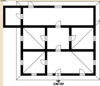
The structure is a load bearing structure in stone. It has a terracotta roof with wooden beam and rafters. The floor is finished with mud.
