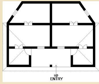
The structure is load bearing in stone and lime with lime plaster. Wooden structure supports the terracotta tiles on the roof.
