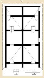
It is a load bearing structure in mud and bamboo. The roof is in wood and terracotta tiles. The floor is laid in mud.
