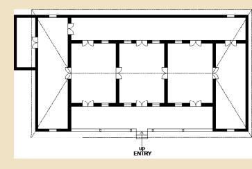
The structure is a load bearing structure in stone and lime. The roof has wooden structure and terracotta tiles. The doors and windows are all in wood. The pillars in the verandah are also wooden. Not at all decorative structure. The aesthetic value of the structure comes from its proportions, roofing and the front pillars in the verandah.
