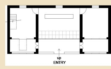
The structure is load bearing in stone, cement, and bricks are also used. The doors and windows are all wooden. The roof has a wooden structure for terracotta tiles for roofing.
