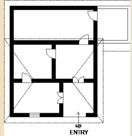
The structure has stone plinth and walls. All peen plastered and white washed. The floor is now cemented and the roof is wooden structure supporting terracotta tiles.
