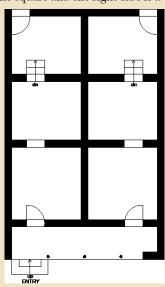
The structure is a load bearing structure in stone, plastered and limewashed in bright pink color. The roof has wooden structure and terracotta tiles.
