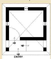
Structure is load bering structure in stone, lime plastered and lime washed. Roof is wooden with terracota tiles  $\frac{1}{2}$
